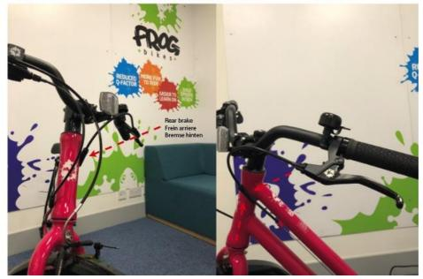
For the European brake setup (i.e., right brake lever is connected with the rear brake), the cable needs to be routed along the right hand side of the head tube (see images for European brake setup below).
