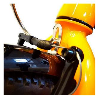
**STEP 1.** Assemble the bits to attach the rear strut to the rear mudguard.
